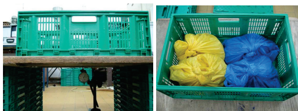
Figure 12 Measuring deformation of the base
