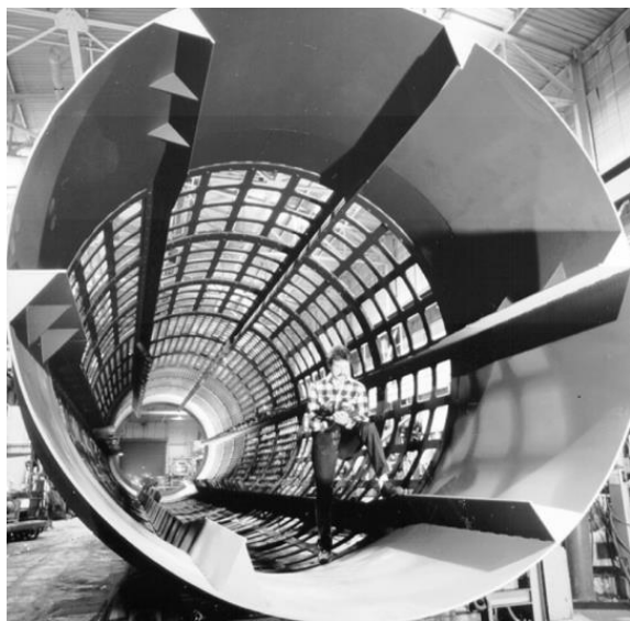
Figure 3. End view of a trommel screen [4]
