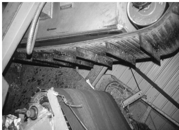
Figure 5. Magnetic belt for separation [4]
