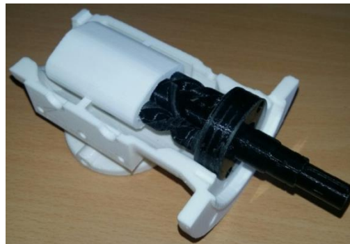
Figure 15. Finished (miniature) 3D model of the assembly of the three-spindle screw pump created by the 3D printer MakerBot Replicator 2X
