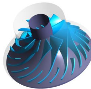
Figure 1 Schematic diagram for the mixed-flow compressor
