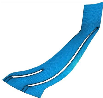
(a) The mesh of one-passage at 60% span
