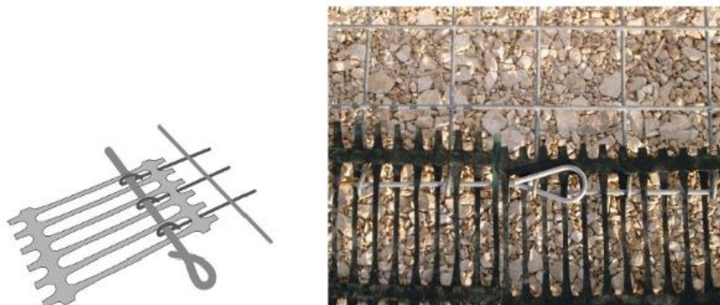
Figure 5 Connection of swaddled steel meshes and geogrids with a bodkin (image source: http://www.tensar.co.uk/ )
