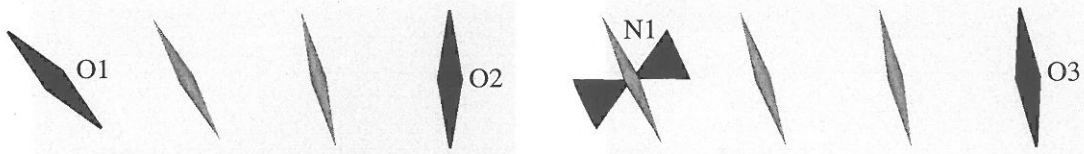
Fig. 4. Two examples of one-dimensional interpolation of orientations. (a) The interpolation is determined based on the given orientations O1 and O2. (b) The interpolation is calculated using the given orientation O3 and normal of orientation N1. The number of iterations amounts to 10.
