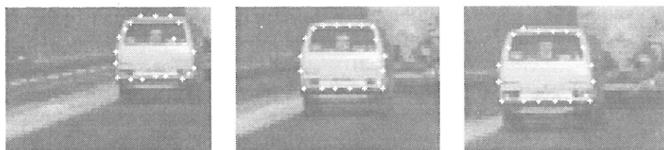
Fig. 8. Results for tracking a car on a highway with active rays (images 4, 44, 84 of a sequence of 123 images taken at video rate): the sampling step size \Delta\phi is \pi/9 .
