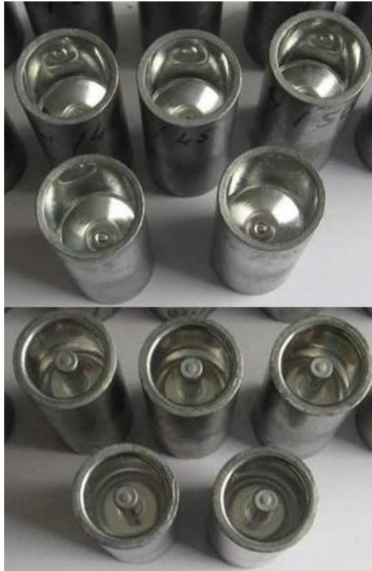
Figure 13: DK-pistons extruded with lubricant 1
