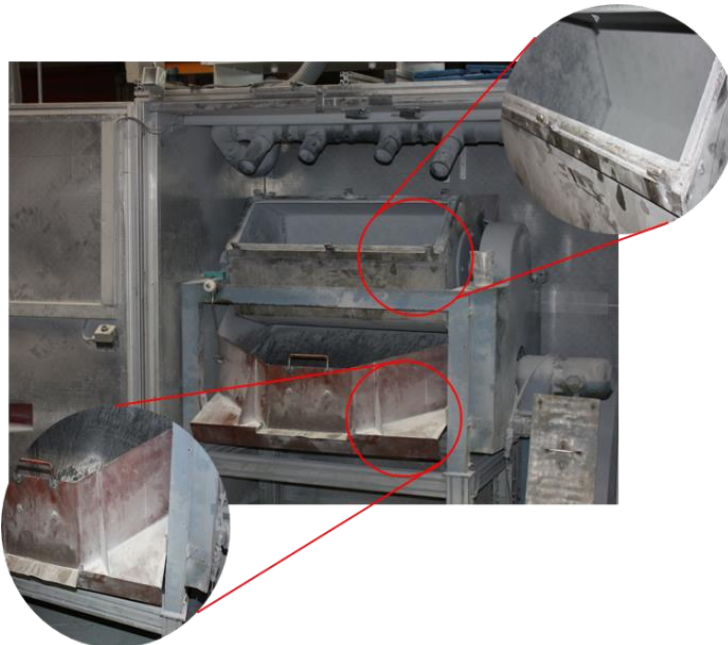
Figure 4: Zinc stearate residues at a tumbler
