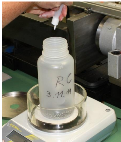
Figure 7: Application of the lubricant dispersion
