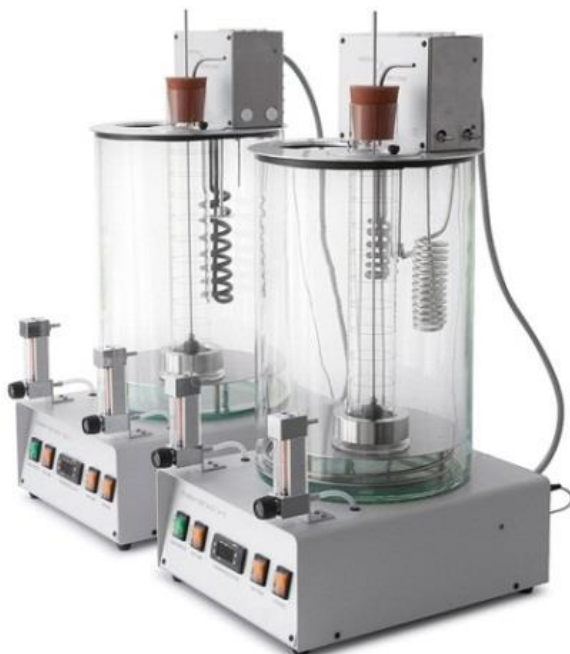
Figure 1: The device for determining the propensity of oil for foaming
