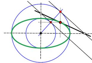
Figure 3: De la Hire’s construction of an ellipse via two orthogonal affinities.
