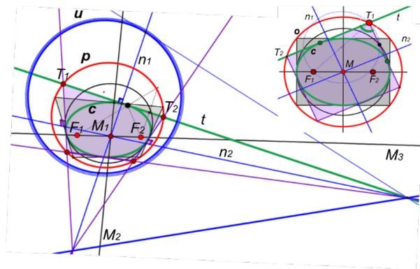
Figure 13: An ellipse  $c$  in a Euclidean or non-Euclidean plane possesses a concentric circle  $p$  containing the vertices of Poncelet quadrangles subscribed to  $c$ .
