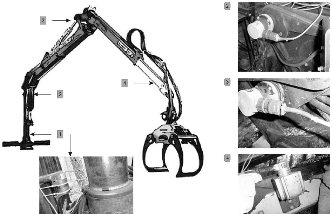
**Fig. 6** Forwarder crane with sensors attached at the joint level for measuring angular motion. This experimental platform has been operating for more than a decade. During this time the sensors have never been changed. Based on this demonstration of the sensing device's reliability and robustness, a commercial version of this solution has been developed (Cranab 2013b)
