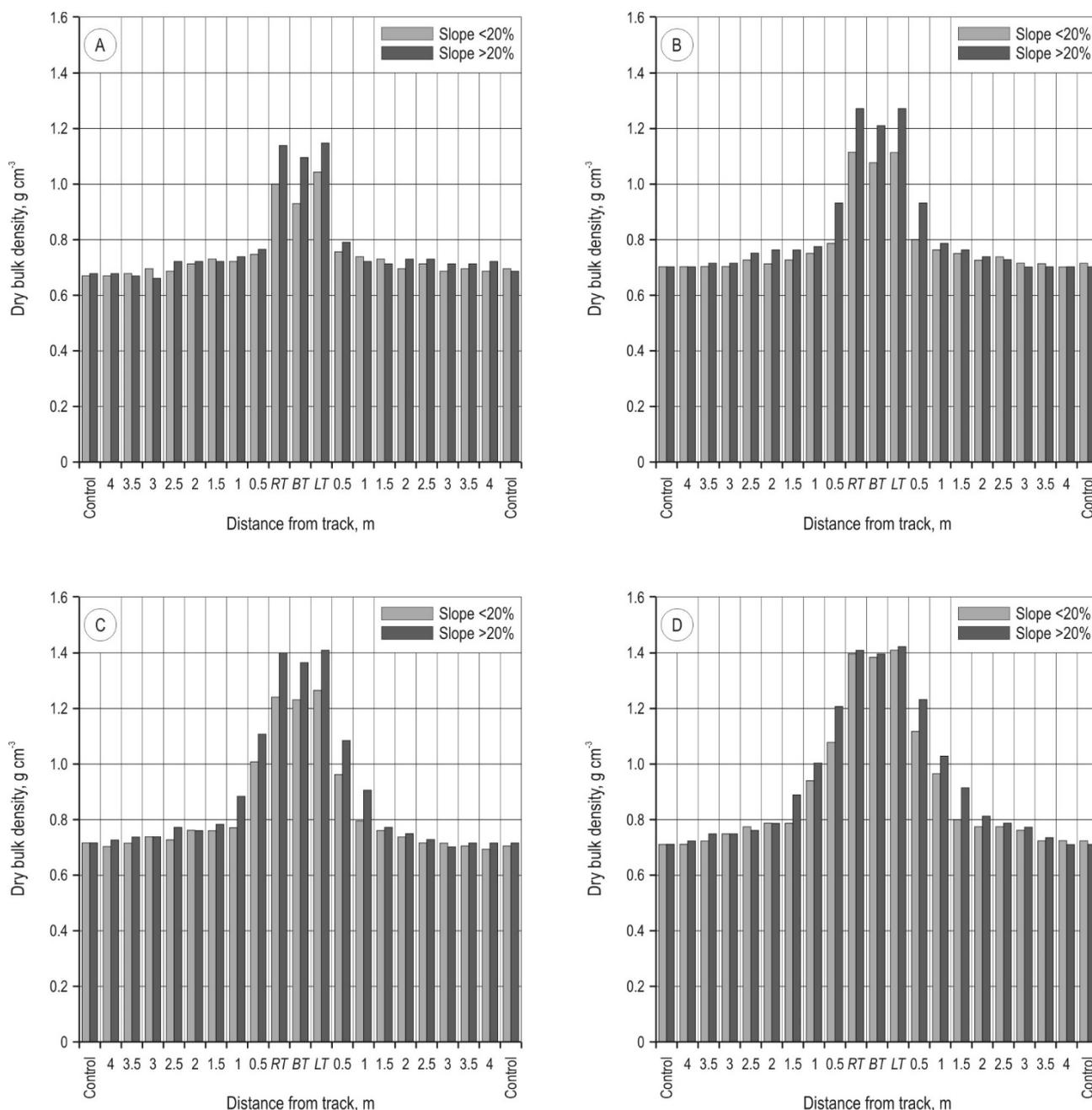
**Fig. 4** Effect of different numbers of skidder passes on soil bulk density under the main track (*LT* and *RT*), log track (*BT*) and at various distances from the end of the track (a: one pass; b: three passes; c: six passes; d: fifteen passes)
