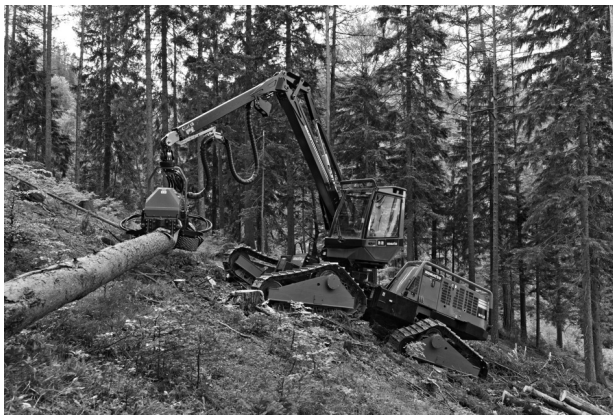
Fig. 3 Komatsu 911.5 X3M, for example, can be fitted with four independently suspended »high-drive« tracks (photo from Komatsu Forest)
