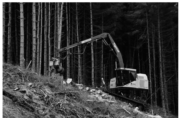
Fig. 2 Tigercat steep terrain feller-buncher shows that self-levelling cab feature is also used to redistribute the weight uphill for increased stability
