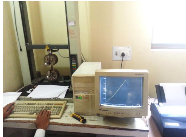
Figure 2. Zwick tensile testing facility.
