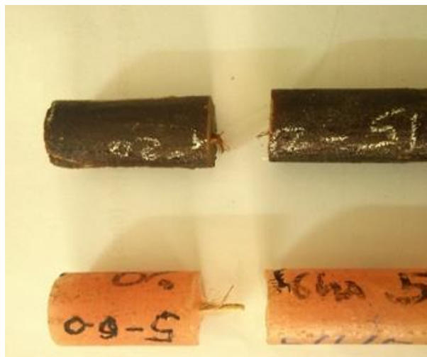
Figure 3. Broken specimens after tensile test.
