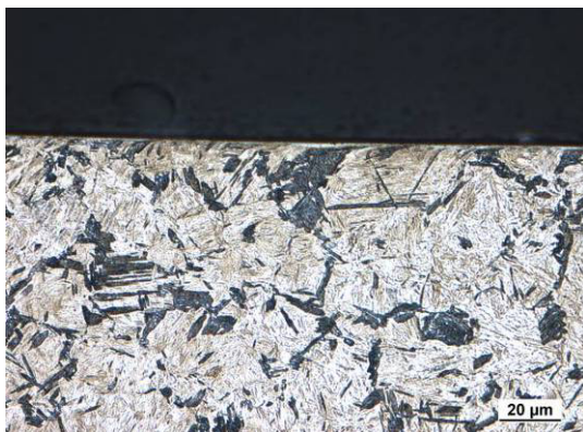
Fig. 2 Microstructure of hard milled surface, VB = 0.05 mm
