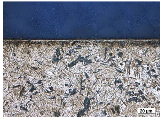
Fig. 3 Microstructure of hard milled surface, VB = 0.4 mm
