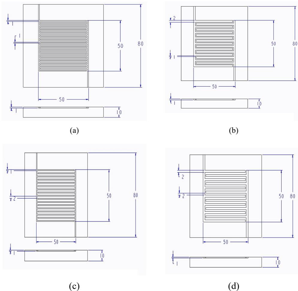
**Fig. 1** Various landing-to-channel width ratios (L: C) (a) 1:1 (b) 1:2 (c) 2:1, and (d) 2:2 of the interdigitated flow channel of 25 cm<sup>2</sup> active area.
