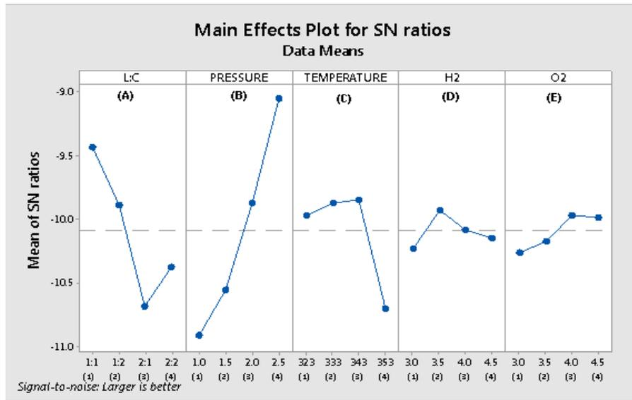
Fig. 3 Mean S/N ratio plot for L: C (A), Pressure (B), Temperature (C), H<sub>2</sub> (D) and O<sub>2</sub> (E)
