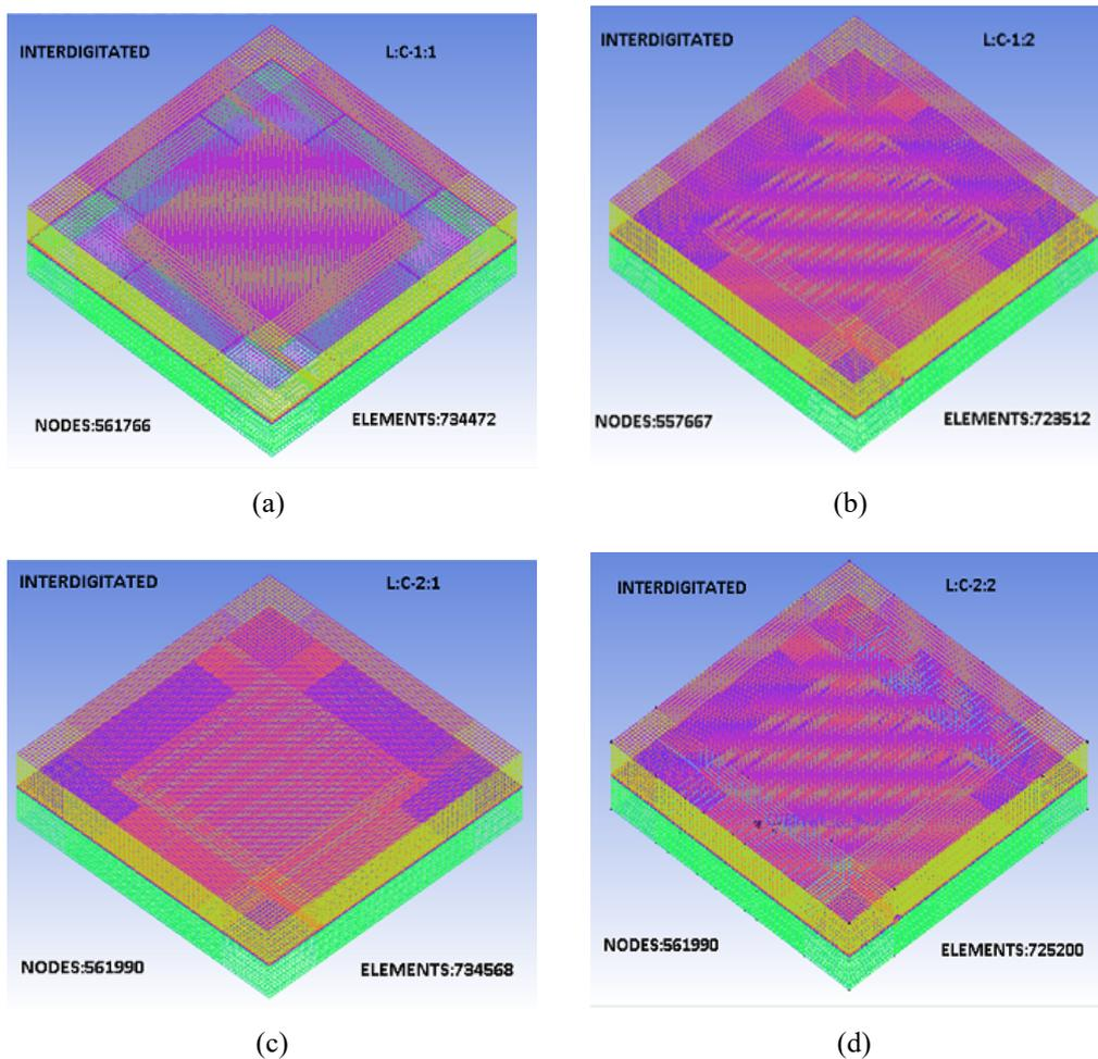
Fig. 2 Meshed assemblies of interdigitated flow channel using ICEM
