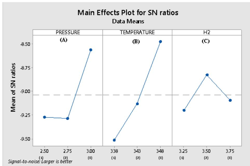
**Fig. 4** Mean S/N ratio plot for refined parameters of Pressure (A), Temperature (B) and H<sub>2</sub> (C)
