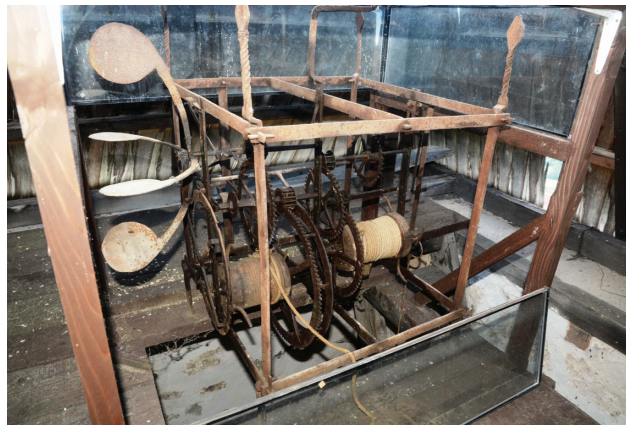
Sl. 2. Satni mehanizam na sahat-kuli u Pruscu Fig. 2. A clockwork mechanism in clock tower in Prusac
