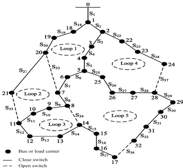
Fig. 3. IEEE 33-bus RDS with state variable sketch
