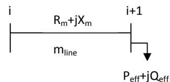
Fig. 2. Single line diagram of a distribution line for loss sensitivity factor
