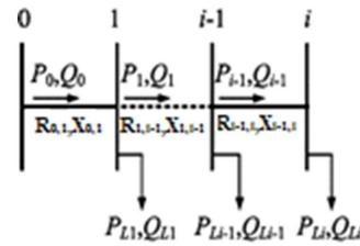
Fig. 1. Single line diagram of a RDS
