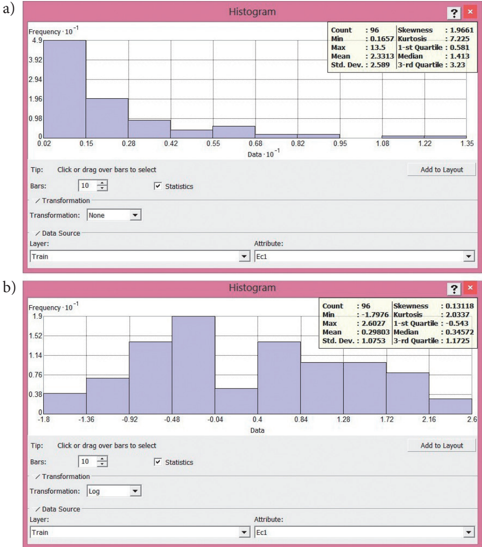
Figure 2. The histograms of training dataset a) before lognormal transformation, b) after lognormal transformation.
