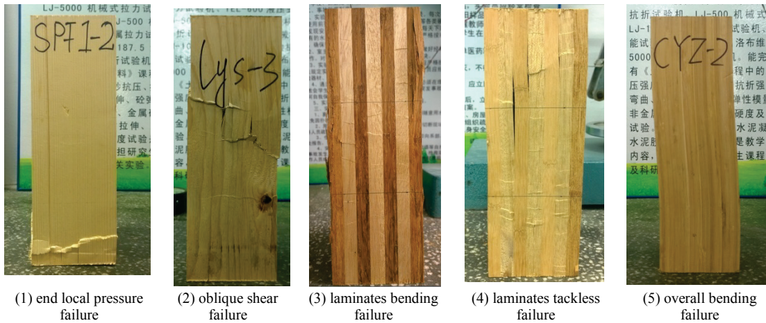
Figure 5 Typical failure modes of the specimens
