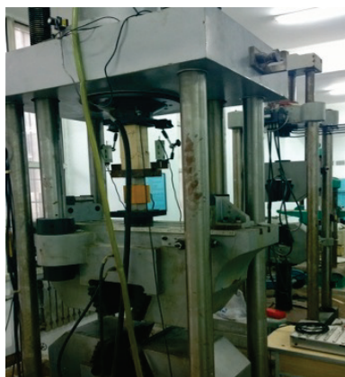
Figure 2 Computer controlled electro-hydraulic servo universal tester
