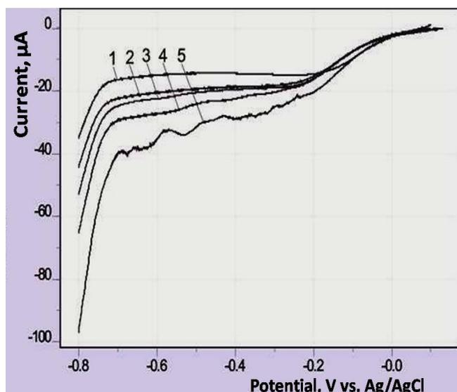
**Figure 3.** Cathodic polarization curves on platinum electrode of electrolyte composition 0.25 M Na<sub>2</sub>MoO<sub>4</sub> at different temperatures: 1 - 295; 2 - 303; 3 - 313; 4 - 323; 5 - 343 K
