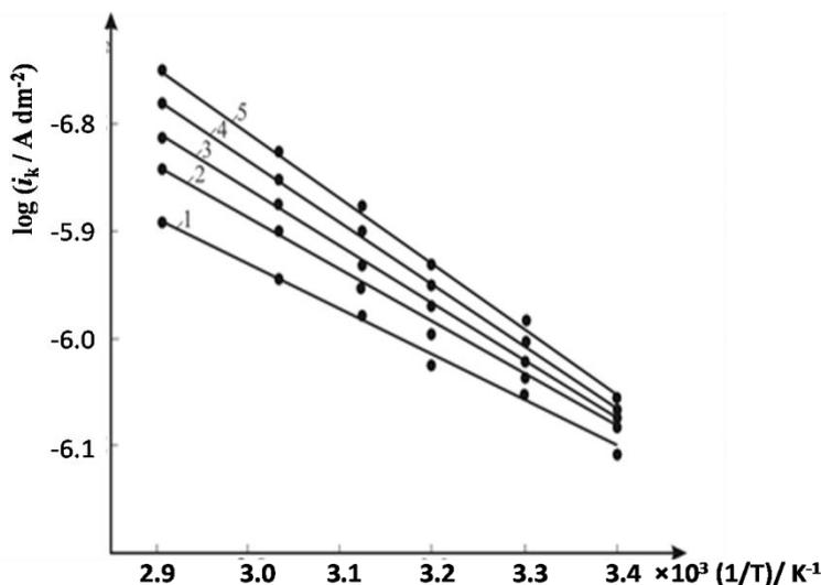
**Figure 4.** Dependence of logarithmic values of the cathodic current density on temperature inverse, the electrolyte consists of -0.25 M Na<sub>2</sub>MoO<sub>4</sub>. At different selected values of potentials vs. Ag/AgCl/KCl<sub>sat</sub>: 1 - 0.2; 2 - 0.4; 3 - 0.5; 4 - 0.6; 5 - 0.7 and 6 - 0.8 V
