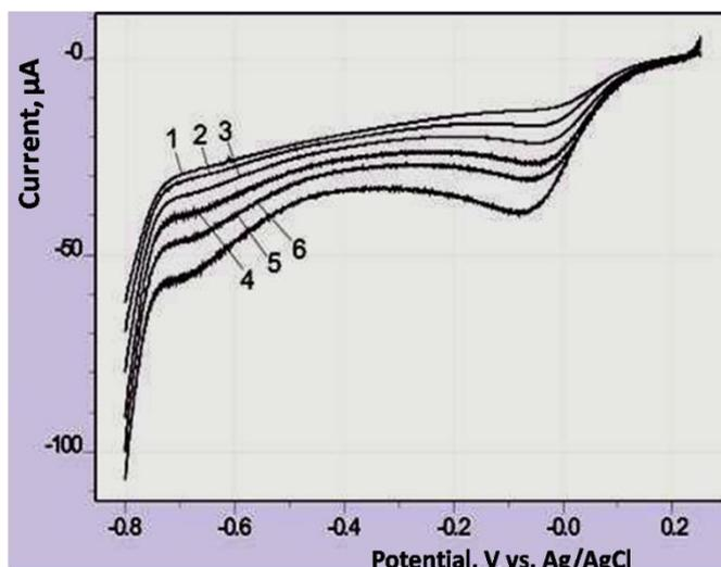
**Figure 1.** Cathodic polarization curves of 0.25 M  $\text{Na}_2\text{MoO}_4$  on platinum electrode at different speed rates of potential: 1 - 5, 2 - 10, 3 - 20, 4 - 40, 5 - 60 and 6 - 80 mV/sec at  $T=295\text{ K}$
