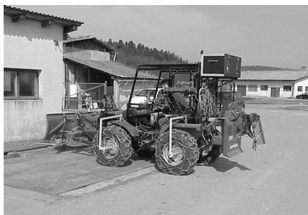
Fig. 1 AGT 835 T tractor prepared for the test
