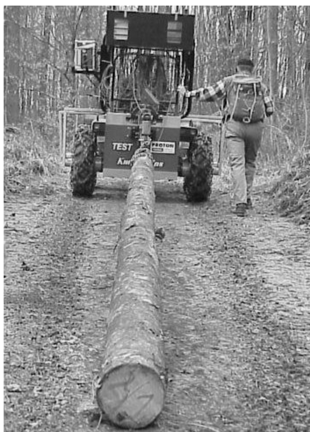
Fig. 2 Skidding at the most steep skid trail
