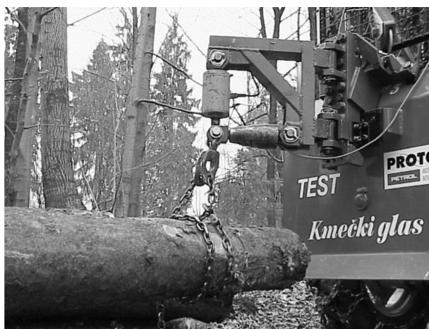
Fig. 5 Measurement of pulling forces on the winch of AGT 835 T
