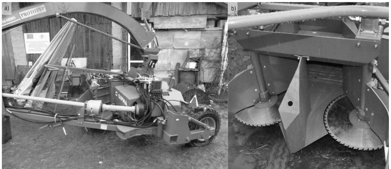
Fig. 17 Prototype of two-row side-operating SIPMA SR 2010 HERO harvester (a) and cutting system (b)
