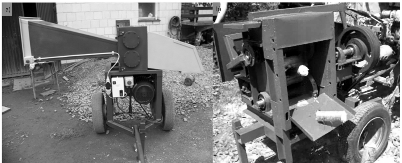
Fig. 14 Prototypes of chipping devices: electric motor-driven (a) and PTO-driven (b)
