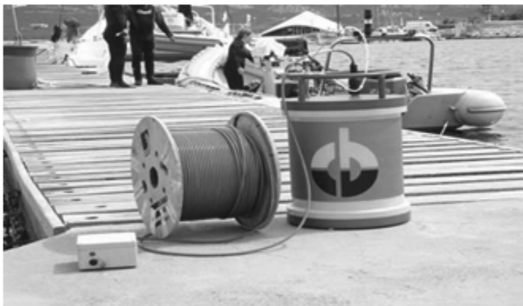
Figure 4 - Buoy equipped for automatic flow cytometry phytoplankton researches [17][18]
