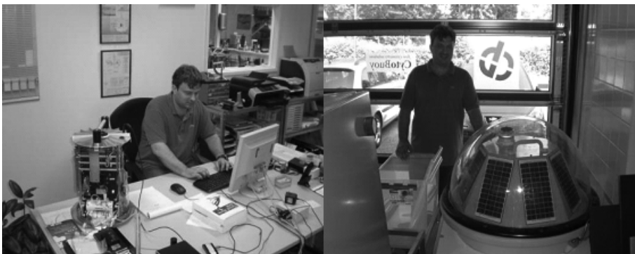
Figure 3 - The buoy and flow cytometer (at the desk, connected to the computer) in the buoy (right side picture)
