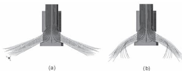
Figure 2 Streamline of molten steel in half SEN: (a) without EMBR; (b) with EMBR
