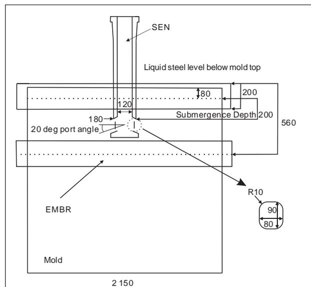
Figure 1 Schematic of the industrial slab caster with two rectangles showing the location of FC-mold electromagnetic brake (all dimensions in mm)
