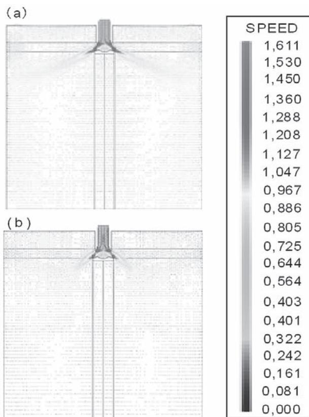
**Figure 4** Velocity field on mold wide face centerplane: (a) without EMBR; (b) with EMBR
