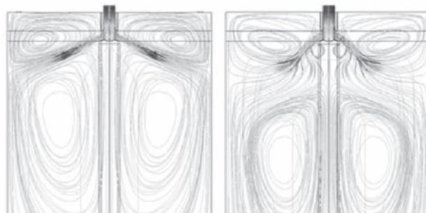
Figure 3 Streamline on mold wide face centerplane: (a) without EMBR; (b) with EMBR
