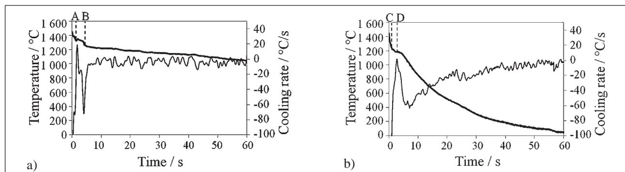
Figure 1 Cooling curves and their derivatives obtained by thermal analysis of CoCrMo alloy. a) Slow cooling and b) fast cooling
