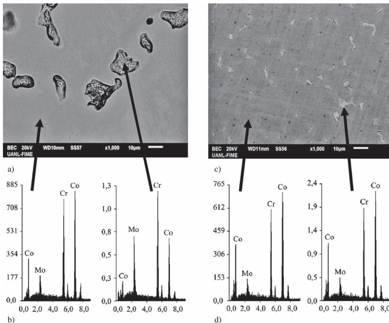
Figure 2 SEM micrographs for both conditions a) slow and c) fast cooling rates, EDS analysis in the Co- $\alpha$  matrix and secondary phases b) slow and d) fast cooling rates
