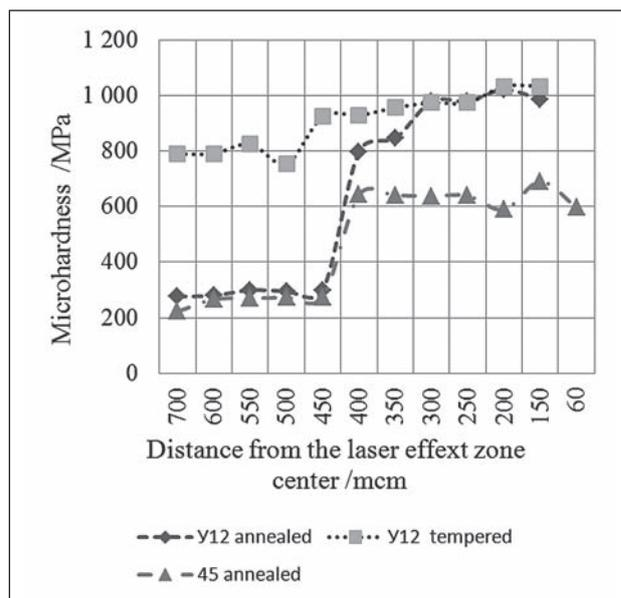
**Figure 4** Microhardness changing in the zone subject to laser treatment with power density 21,8 kW/cm<sup>2</sup>
