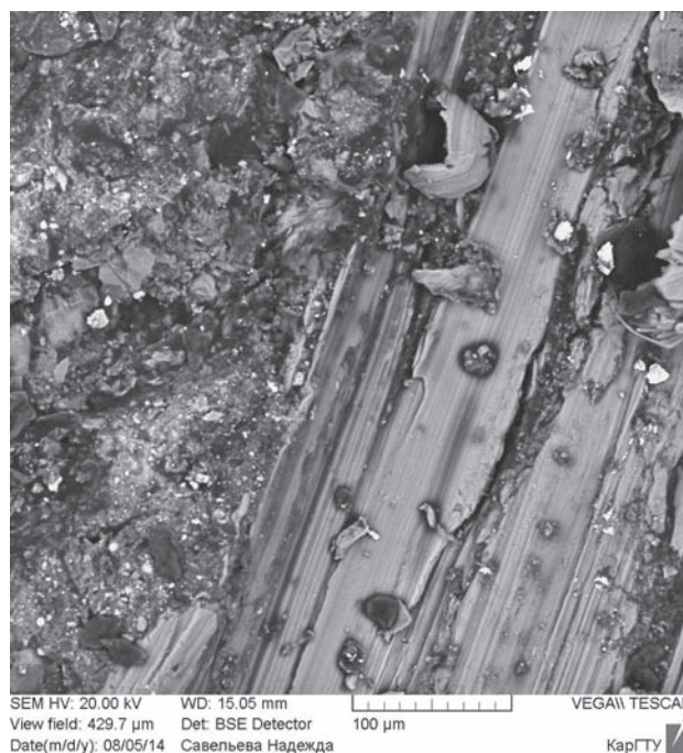
Figure 7 Coating-substrate transfer at x 800 fold magnification
