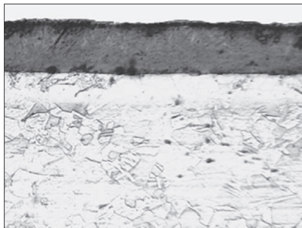
Figure 2 Microstructure of nitrided steel 304L, etching-glycergia, 240x
