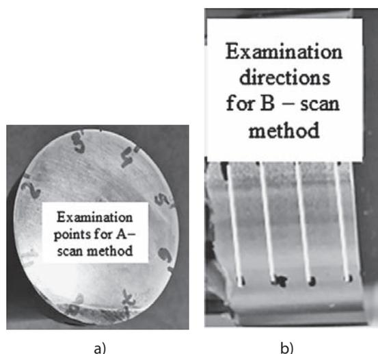
Figure 2 Ultrasonic testing areas: a - A-scan, b - B-scan
