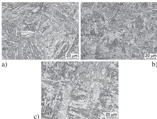
**Figure 1** Microstructure of the joint subjected to PWHT: a) PB2 steel parent metal: tempered martensite; b) coarse-grained HAZ (CGHAZ): tempered martensite; c) weld: tempered martensite; etchant:  $\text{FeCl}_3$ , mag. 500x
