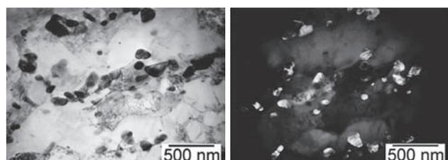
**Figure 6** Morphology of  $M_{23}C_6$  carbides observed in the CGHAZ area of the joint welded using the TBT: a) bright visual field; b) dark visual field; c) SAED diffraction pattern of  $M_{23}C_6$  carbides:  $112_{\alpha} \parallel [013]_{M_{23}C_6}$
