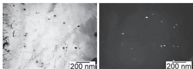
**Figure 7** Morphology of NbC carbides observed in the CGHAZ area of the joint welded using the TBT: a) bright visual field; b) dark visual field; c) SAED diffraction pattern of NbC carbides
