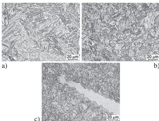
**Figure 2** Microstructure of the joint not subjected to PWHT, i.e. welded using the TBT: a) PB2 steel parent metal: tempered martensite; b) CGHAZ: tempered martensite; c) weld: tempered martensite + delta ferrite; etchant:  $\text{FeCl}_3$ , mag. 500x
