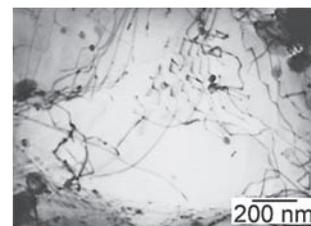
served  $M_{23}C_6$ , NbC and V(CN) carbide particles are presented in Figures 5–8. The size of the MX-type fine/dispersive precipitates was restricted within the 10–40 nm range.
