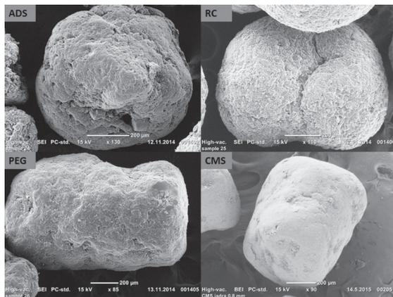
Fig. 2. SEM images of cores.
