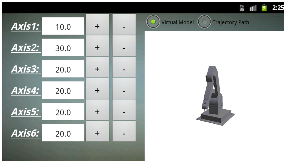
Fig. 7. Remote robot control in manual mode with monitoring using 3D robot model
