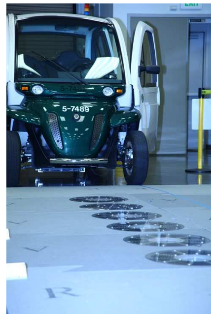
Fig. 6. In motion wireless charging system for electric vehicle application "used with permission of ORNL" [107]
