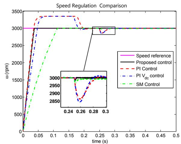
Fig. 19. Speed regulation comparison of the proposed, PI and SM controllers at  $\omega_r = 3000 \text{ rpm}$ ,  $T_{load} = 3 \text{ N.m}$  applied at 0.25 s, motor M1
