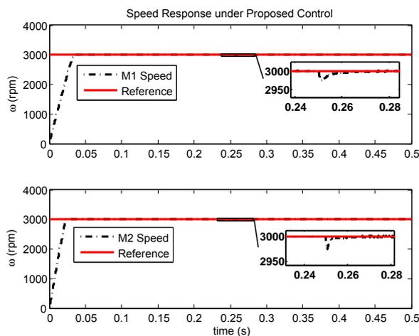
Fig. 13. Speed regulation response with proposed controller for M1 and M2 under  $\omega_r = 3000$  rpm and rated load
