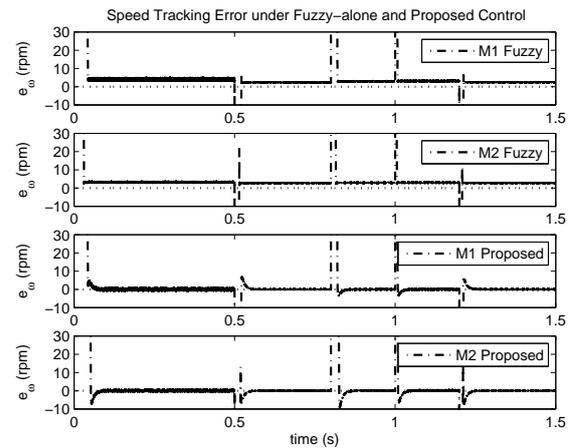
Fig. 18. Speed tracking error comparison between fuzzy and proposed controllers for M1 and M2 under constant load
