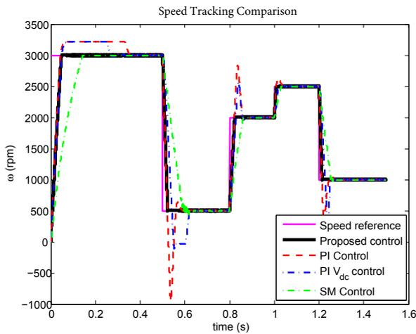
Fig. 20. Speed tracking comparison of the proposed, PI and SM controllers under constant  $T_{load} = 1.5 \text{ N.m}$ , motor M1
