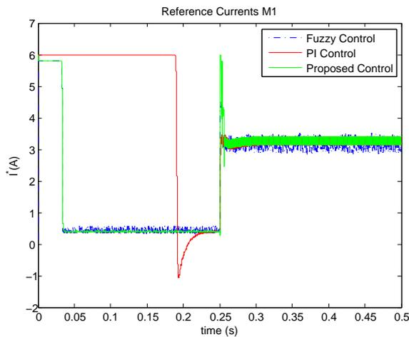
Fig. 21. Reference current  $I^*$  for M1 under the fuzzy alone, PI and the proposed control schemes at a set-point speed of 3000 rpm and  $T_{load} = 3 \text{ N.m}$  applied at 0.25 s
