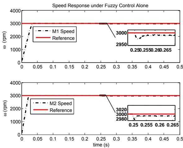
Fig. 12. Speed regulation response with fuzzy logic controller alone for M1 and M2 under  $\omega_r = 3000$  rpm and rated load
