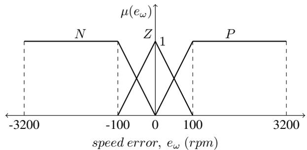
Fig. 5. Input  $e_\omega$  membership functions, motor M2
