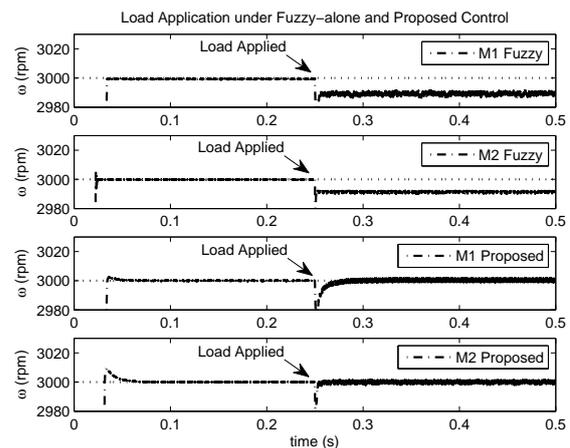
Fig. 15. Speed regulation comparison (zoomed view) between fuzzy and proposed controllers under  $\omega_r = 3000$  rpm and rated load
