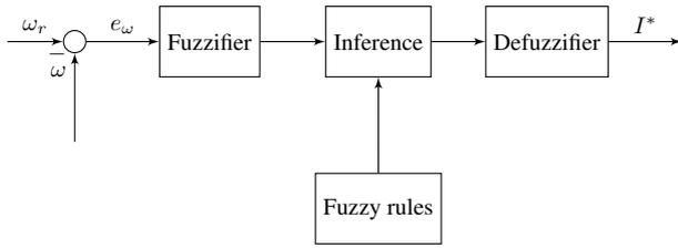
Fig. 2. Fuzzy controller block diagram
