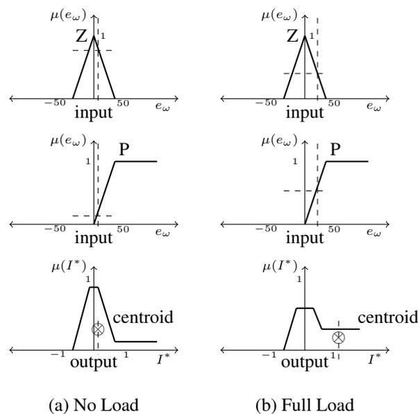
Fig. 9. Input fuzzy sets (top and middle rows), output fuzzy sets (bottom row) and centroid locations under no–load and full load at rated speed
