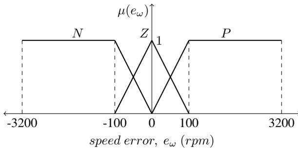
Fig. 3. Input  $e_\omega$  membership functions, motor M1
