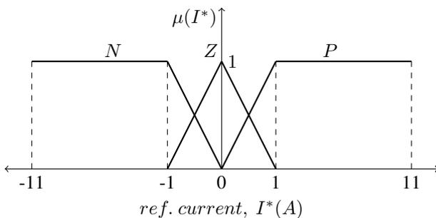
Fig. 4. Output  $I^*$  membership functions motor M1
