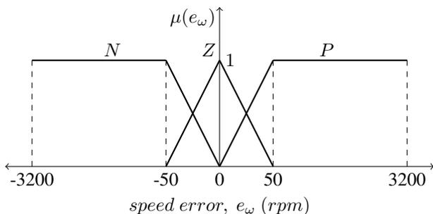
Fig. 7. Modified Input  $e_{\omega}$  membership functions, motor M1 with increased slopes
