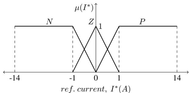
Fig. 6. Output  $I^*$  membership functions motor M2
