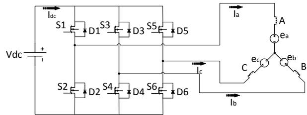
Fig. 1. A simplified BLDC motor drive
