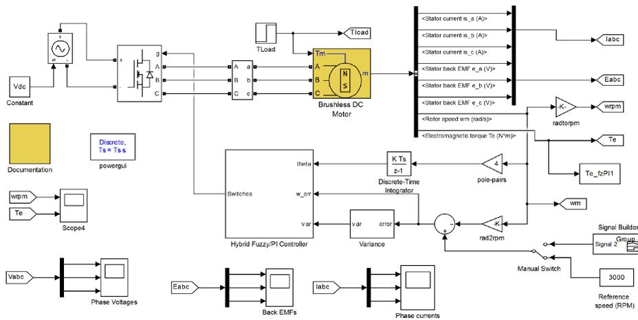
Fig. 11. Simulink model of the hybrid Fuzzy/PI speed control system
