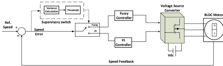
Fig. 10. Simplified block diagram of the drive system under proposed control
