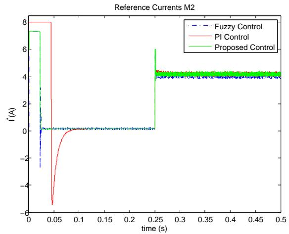
Fig. 22. Reference current  $I^*$  for M2 under the fuzzy alone, PI and the proposed control schemes at a set-point speed of 3000 rpm and  $T_{load} = 1.91 \text{ N.m}$  applied at 0.25 s
