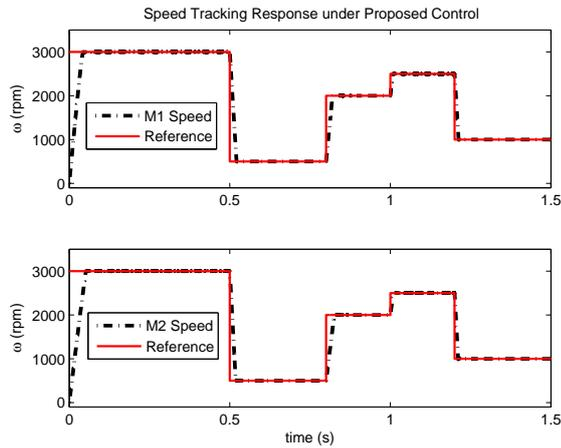
Fig. 17. Speed tracking response of proposed controller, for M1 and M2 under constant load
