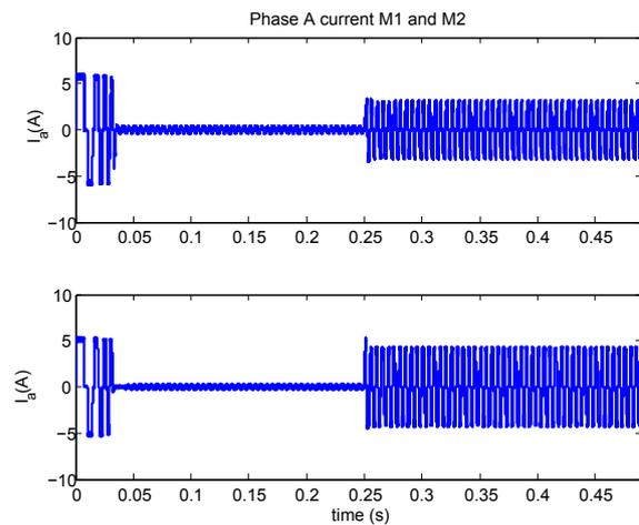
Fig. 23. Phase A currents of M1 and M2 under proposed scheme for a set-point speed of 3000 rpm,  $T_{load} = 3 \text{ N.m}$  for M1 and  $T_{load} = 1.91 \text{ N.m}$  for M2 applied at 0.25 s
