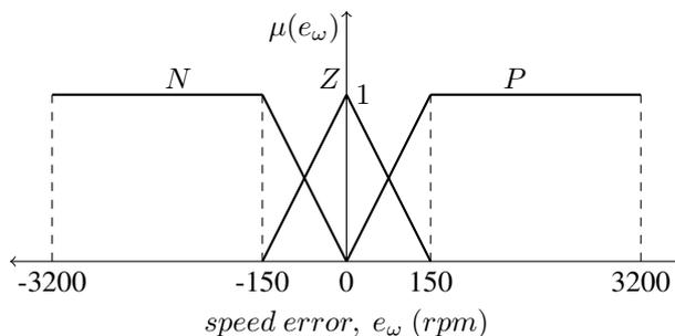
Fig. 8. Modified Input  $e_{\omega}$  membership functions, motor M1 with reduced slopes
