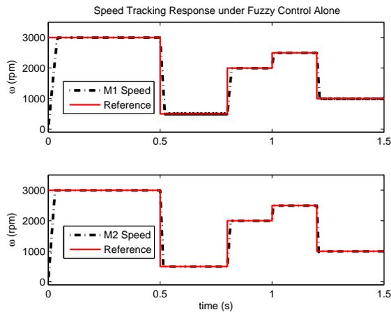
Fig. 16. Speed tracking response of fuzzy logic controller alone, for M1 and M2 under constant load
