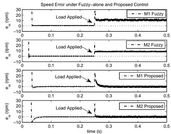
Fig. 14. Speed regulation error comparison between fuzzy and proposed controllers under  $\omega_r = 3000$  rpm and rated load
