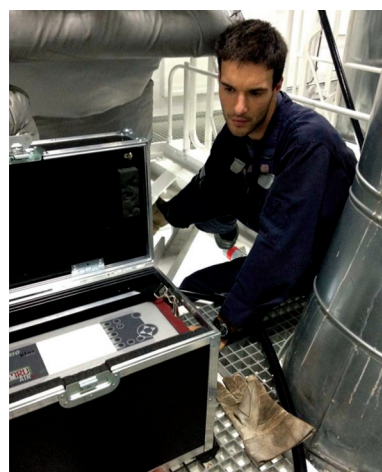
Figure 3 Measuring exhaust emission on Mak 9M 32C engine with MRU
