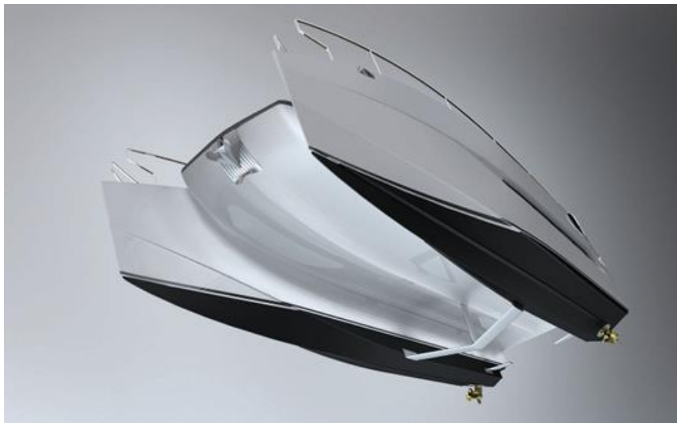
Fig. 1 Foil between catamaran hulls
