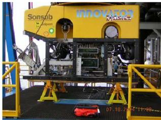
*Figure 2. Sonsub Innovator workclass (yellow) and Seabotix miniclass ROV (red)*
