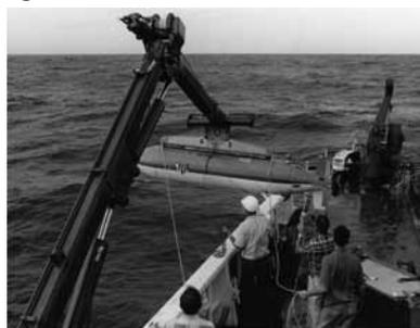
*Figure 4. SPURV II in launch.*
