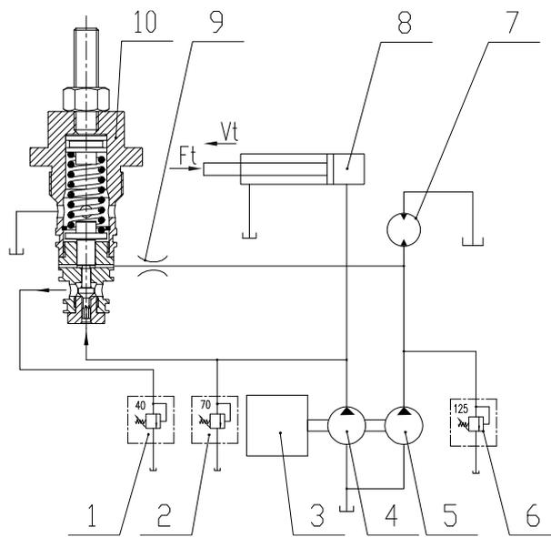
Figure 1. Schematic diagram of anti-jamming system. 1-low feed pressure relief valve; 2-high feed pressure relief valve; 3-engine; 4-feed pump; 5- rotation pump; 6-rotation relief valve; 7-rotary motor; 8-feed cylinder;9-damper orifice; 10-anti-jamming valve.
