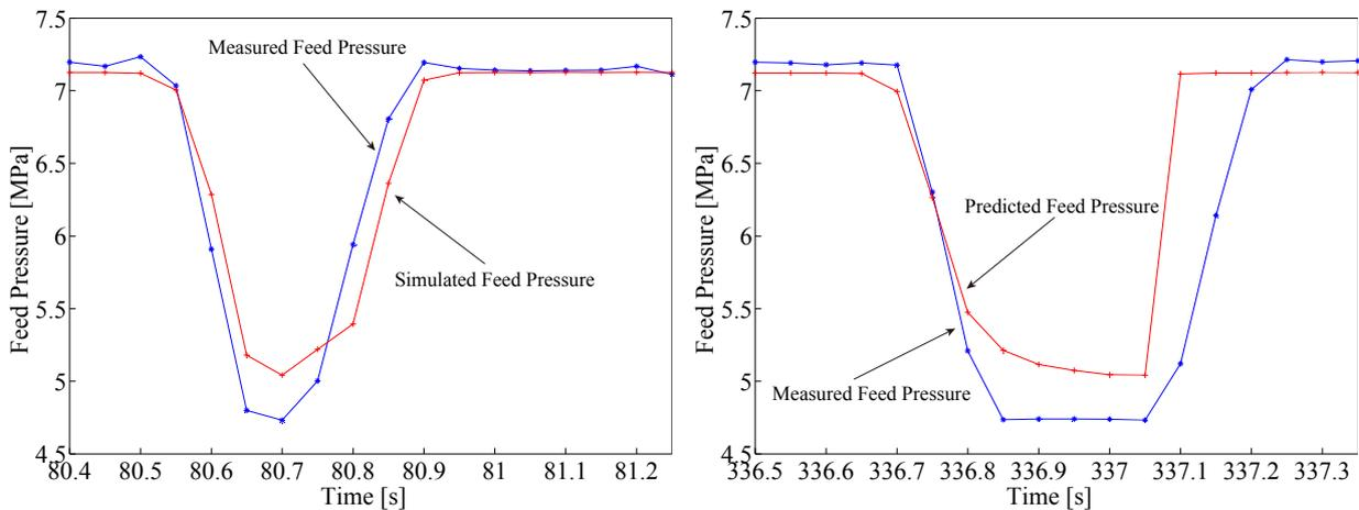
Figure 7. Simulation and prediction of feed pressure (1 hidden node).
