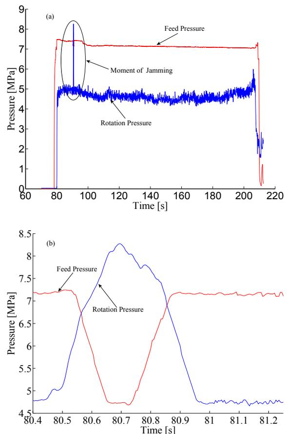
Figure 4. Curves of feed and rotation pressure:
