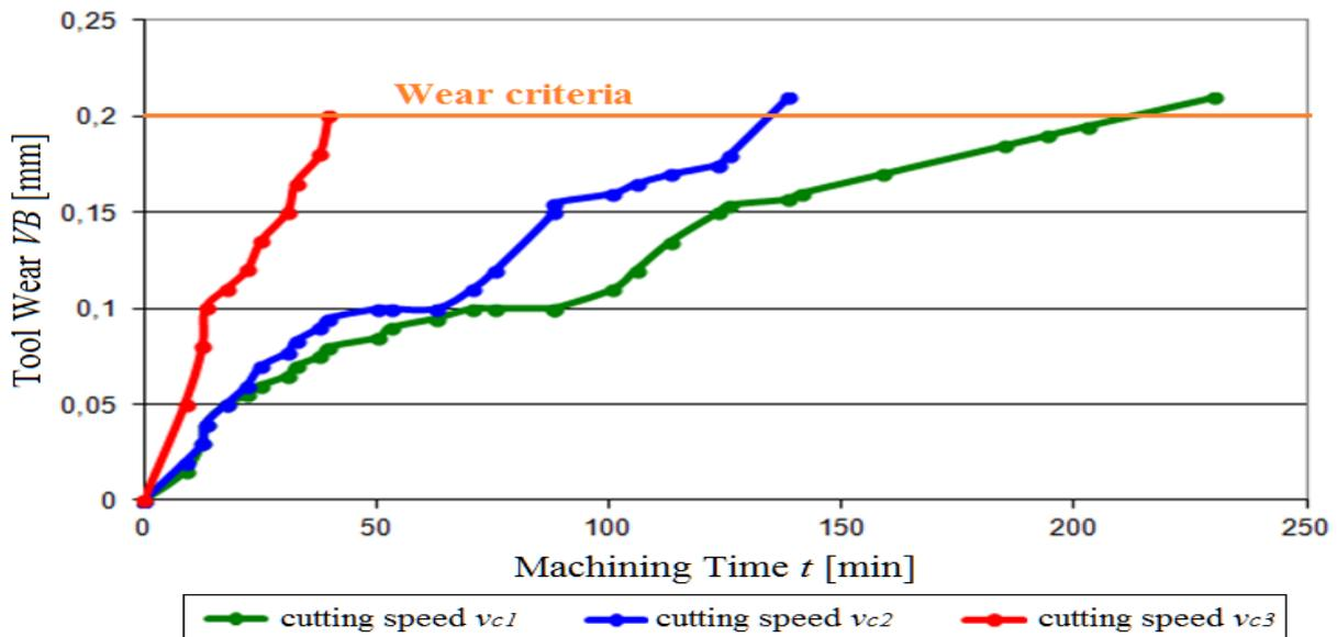
Figure 5. Graphical presentation of dependence of tool wear on machining time in rough milling of Hardox 500 steel with cemented carbide cutting tool inserts to determine the dependence of  $T = f(v_c)$ .
