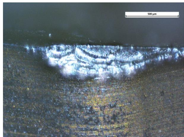
Figure 4. Surface morphology of worn cutting insert investigated with optical microscope Nikon Eclipse LV100ND (50x).
