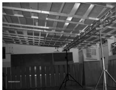
Figure 2. The auxiliary framing and covering plates in the test room
