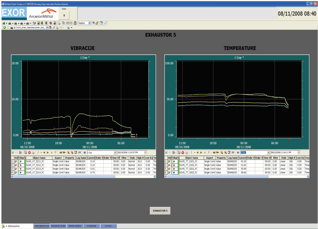
Figure 5 Vibrations and temperatures on four slide bearings on process fan 5 during one day
