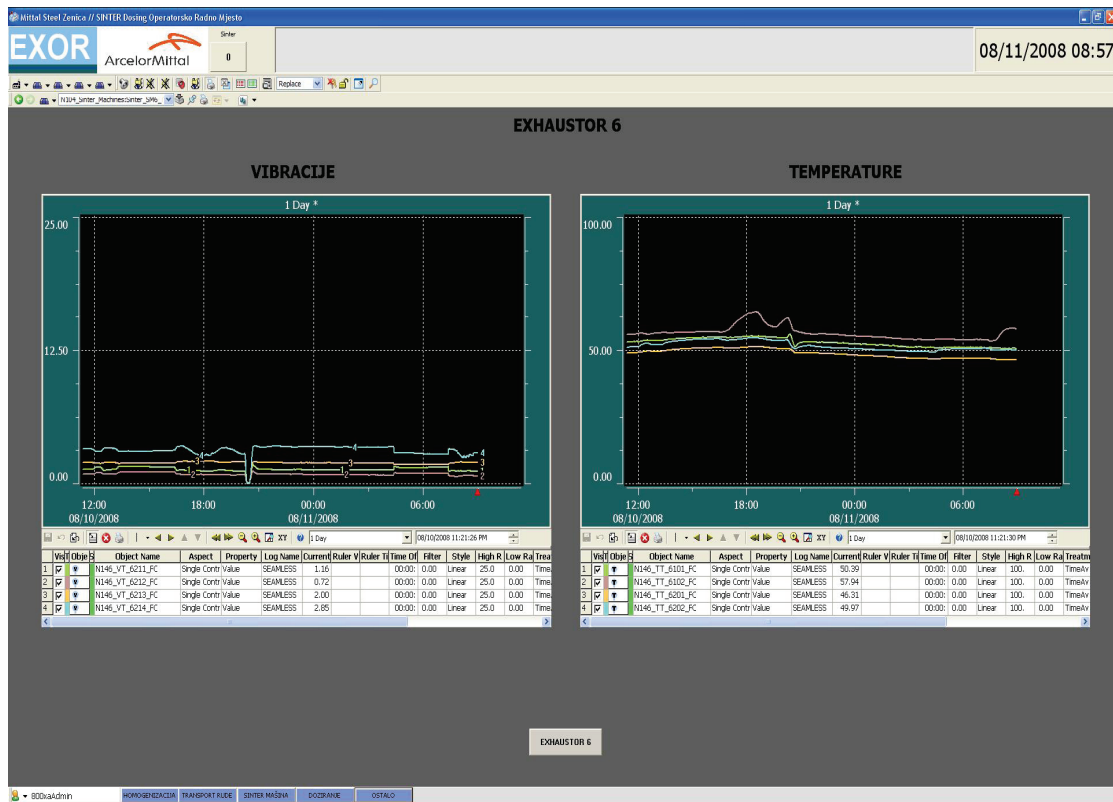
Figure 6 Vibrations and temperatures on four slide bearings on process fan 6 during one day
