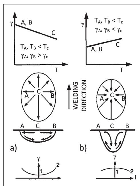
**Figure 1** Heiple-Roper model for Marangoni convection in weld pool (a) low sulfur steel and (b) high sulfur steel [5]
