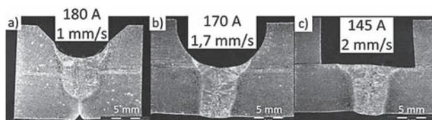
**Figure 5** Macrosections of A-TIG welds on 10 mm plate with a) V groove, b) U groove and c) flat groove
