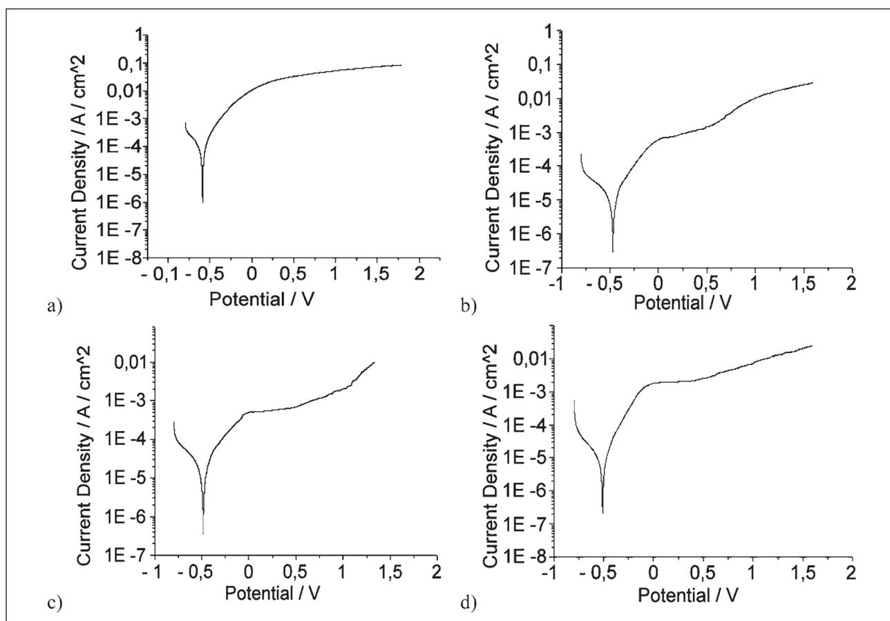
**Figure 5** Voltammetric characteristics for: a - HS6-5-2 steel and b) a - C:H:W; c) CrN/a - C: H: W; d) TiN/a - C:H:W coatings
