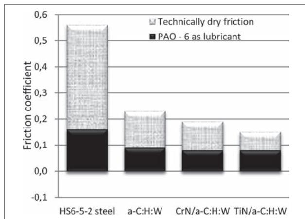
**Figure 4** The friction coefficients obtained for the tested materials.
