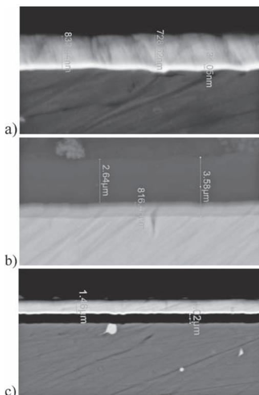
**Figure 3** SEM microstructure of the cross-sectional measurement of the coating thickness: a) a - C:H:W, b) CrN/a - C:H:W, c) TiN/a - C:H:W
