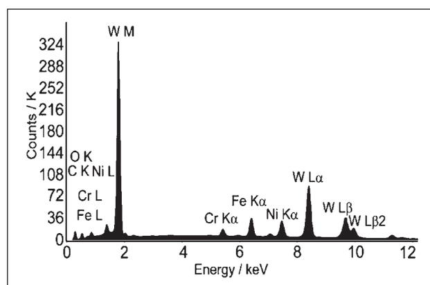
**Figure 2** The EDS point analysis of elemental composition of a - C:H:W coating
