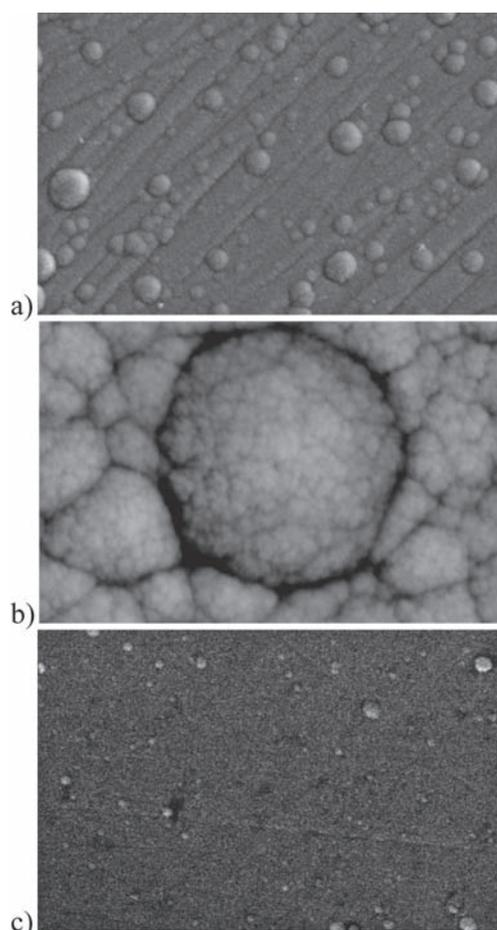
**Figure 1** SEM - images of the surface of diamond - like coatings: a) a - C:H:W, b) CrN/a - C:H:W, c) TiN/a - C:H:W
