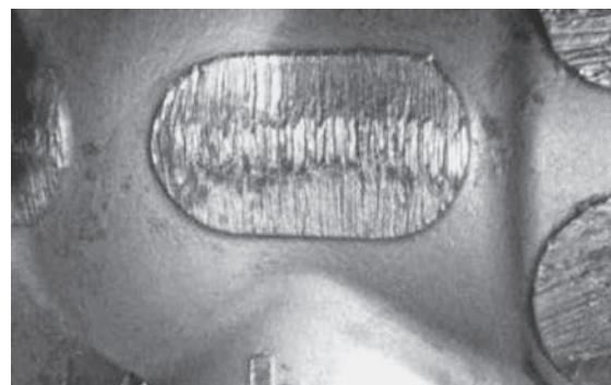
Figure 4 Representation of a clean casting without defects
