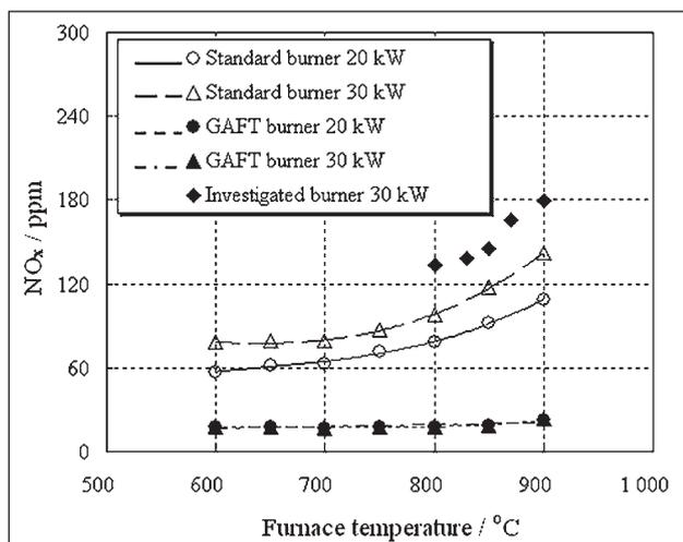
**Figure 1** Effects of the furnace temperature on  $\text{NO}_x$  emission from the U radiant tube for  $l = 1,1$
