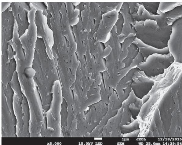
Figure 5 Microcracks in the grain area of the modified cast steel – 60 °C
