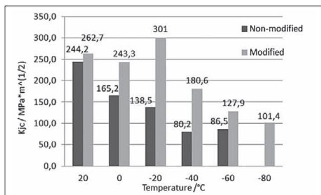
**Figure 2** Cracking resistance,  $K_{Ic}$ , for G17CrMo5-5 cast steel
