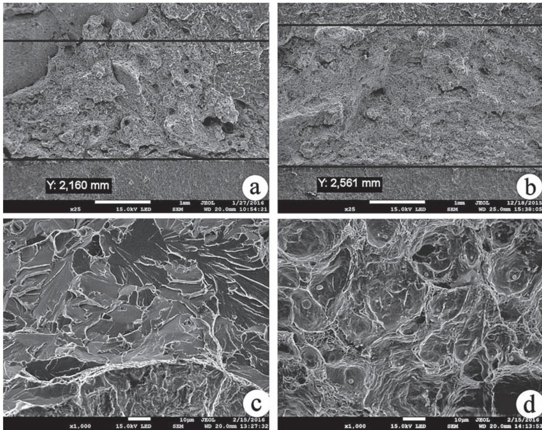
Figure 3 Fracture surface under the notch bottom: a,c – non modified, b,d – modified
