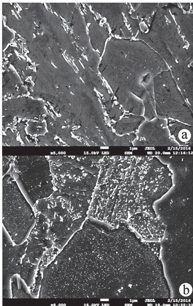
**Figure 1** Microstructure of G17CrMo5-5 cast steel: a – non-modified, b – modified, scanning electron microscopy image
