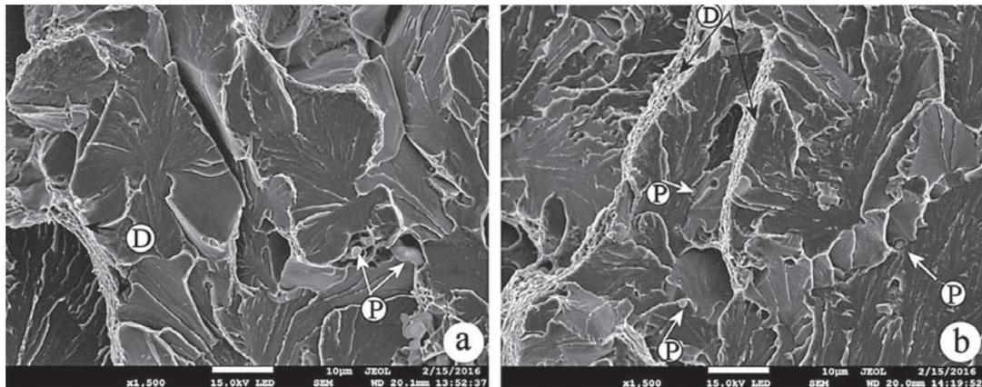
Figure 4 Brittle fracture surface: a – non-modified, b – modified (– 40 °C)
