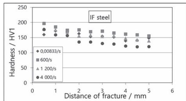
**Figure 4** Effect of hardness HV1 on the distance from the quarry at different strain rates IF steel
