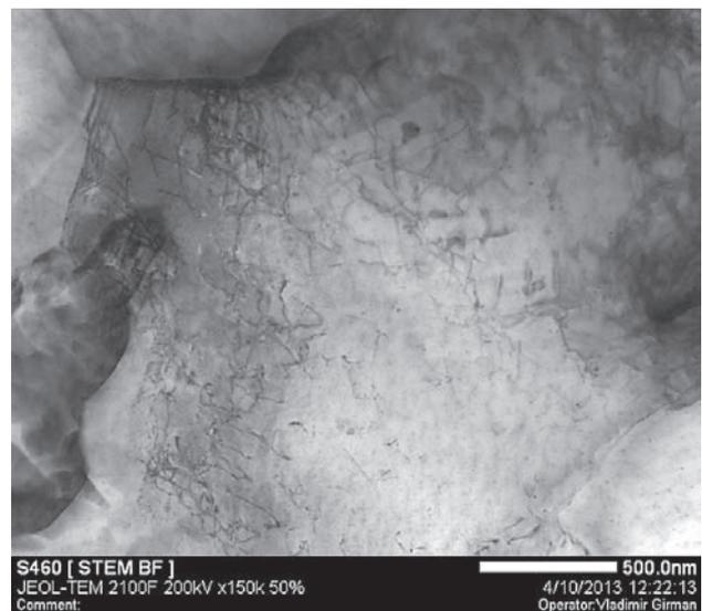
**Figure 9** Dislocation structure of S420 steel in the static condition ( $\dot{\epsilon} = 3\,000 \cdot s^{-1}$ )
