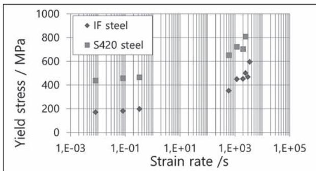
**Figure 2** Dependence strain rate of IF and S420 steel sheets stress
