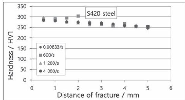
**Figure 5** Effect of hardness HV1 on the distance from the quarry at different strain rates S420 steel
