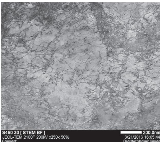
**Figure 8** Dislocation structure of S420 steel in the static condition ( $\dot{\epsilon} = 8,33 \cdot 10^{-4} \cdot s^{-1}$ )
