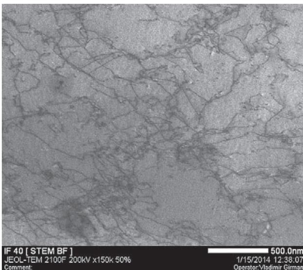
**Figure 7** Dislocation structure of IF steel in the dynamic condition ( $\dot{\epsilon} = 4\,000 \cdot s^{-1}$ )
