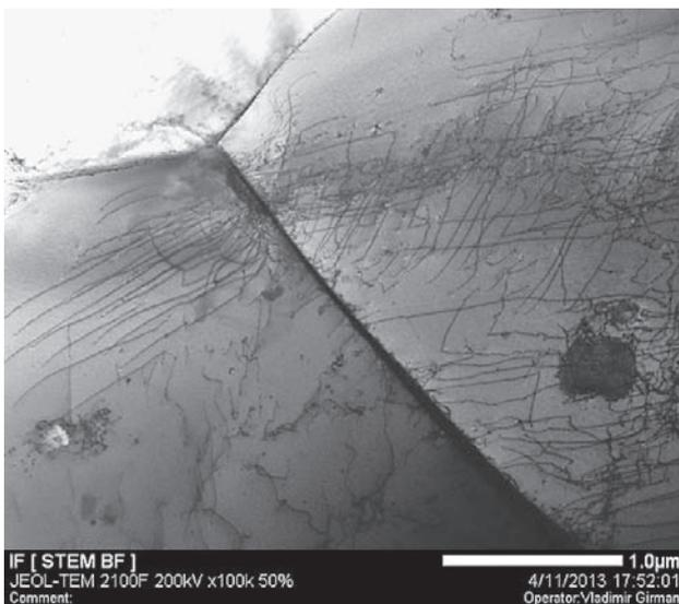
**Figure 6** Dislocation structure of IF steel in the static condition ( $\dot{\epsilon} = 8,33 \cdot 10^{-4} \cdot s^{-1}$ )
