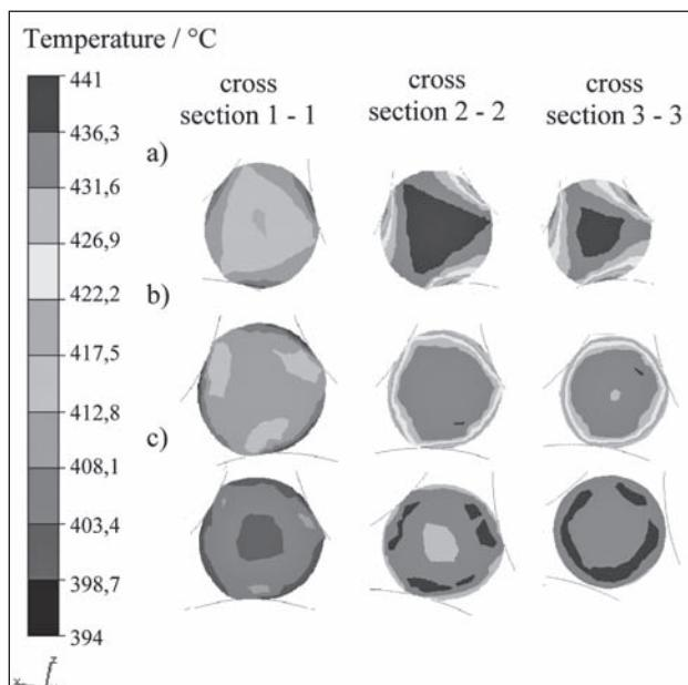
**Figure 4** Temperature distributions in cross-sections of the rolled bar during the rolling of ingot with diameter of  $\phi 26$  mm to the bar with diameter of  $\phi 24$  mm with temperature of  $400$  °C and rotational speed of the rolls of: a)  $n_w = 25$  rev/min, b)  $n_w = 75$  rev/min, c)  $n_w = 100$  rev/min
