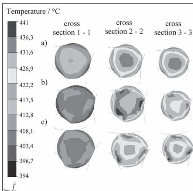
**Figure 3** Temperature distributions in cross-sections of the rolled bar during the rolling of ingot with diameter of  $\phi 30$  mm to the bar with diameter of  $\phi 26$  mm with temperature of  $400$  °C and rotational speed of the rolls of: a)  $n_w = 25$  rev/min, b)  $n_w = 75$  rev/min, c)  $n_w = 100$  rev/min
