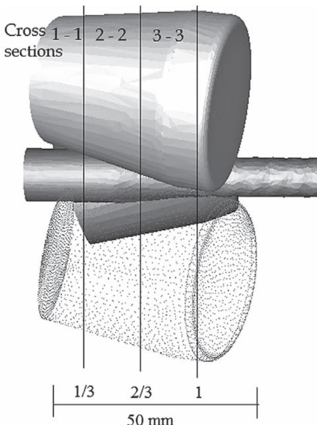
**Figure 2** The cross-sections in which the temperature distributions in deformed bars were analyzed
