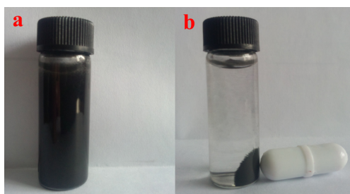
Figure 6. Typical photographs of dispersed nanostructures in solution (a) and after using a magnetic field (b)
